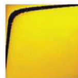
F-7B Brass Mirror polished face, dark edges
